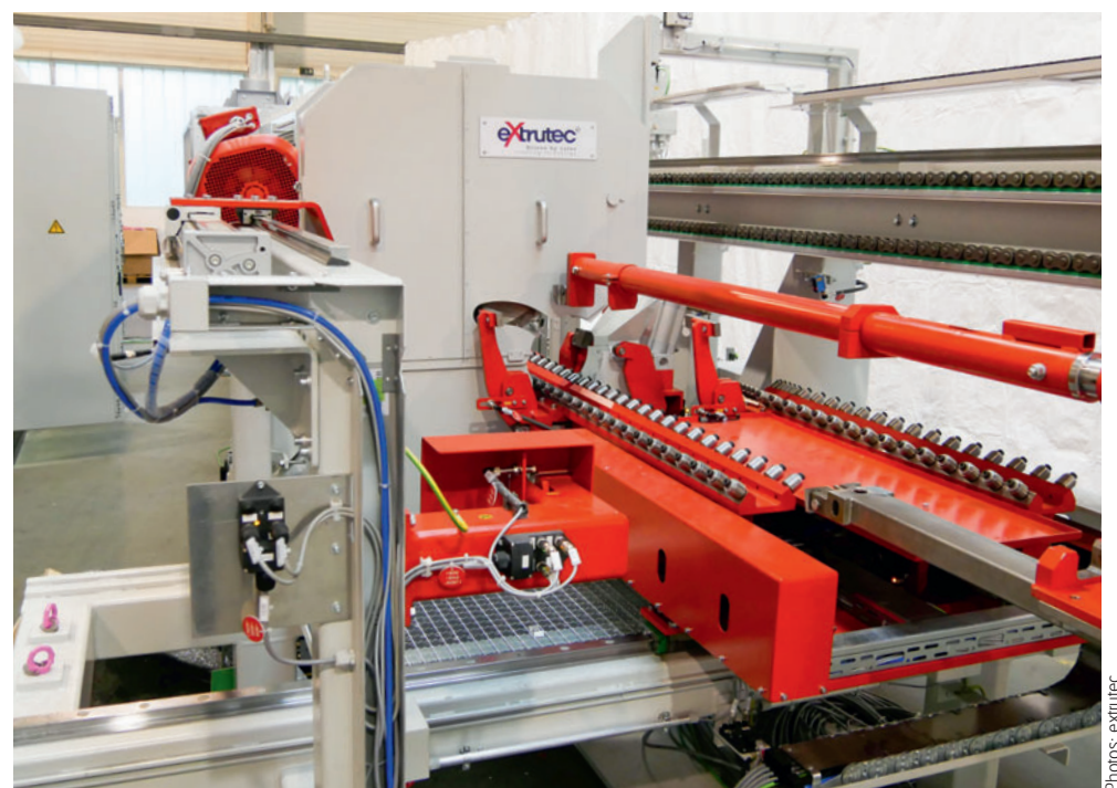
Detailed view of a new 8-inch hot saw for logs with billet cross transfer
