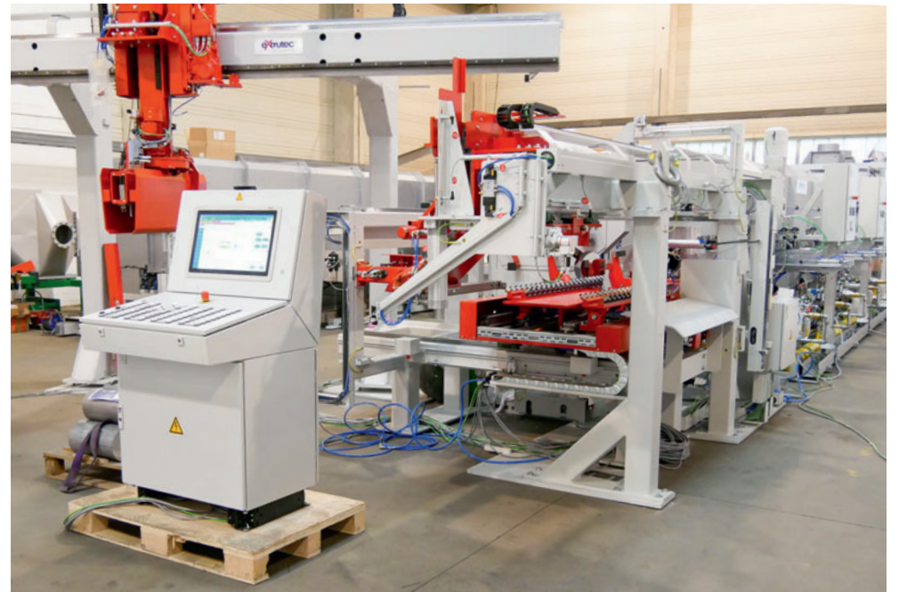
New 8-inch extrutec in-line furnace unit (patented) with a hot saw for logs and a billet manipulator
