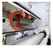
the gas heater, the aluminium logs are pre-heated to temperatures of up to 90 °C by laminar water flow of the entire surface with hot water. It is another pioneering result for the benefit of our customers and for sustainable protection of our environment.
