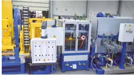
This photo shows an IAS induction heater installed directly after the extrutec gas heater in patented 'in-line' configuration during workshop assembly.
