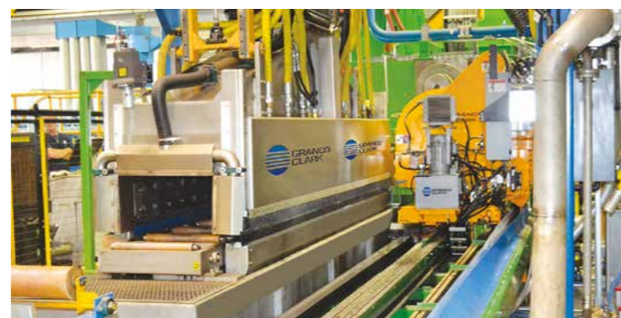
Granco Clark's pull-through quench pulls the extrusion through the operating quench environment without first-billet scrap.
