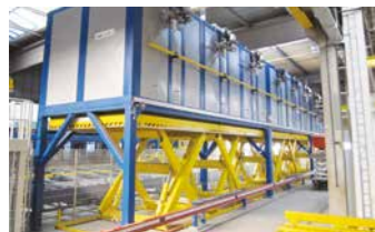
extrutec ageing oven system in overhead arrangement.
