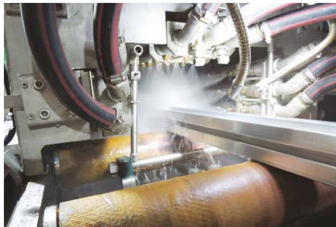
Front view of water quenching section during operation.
